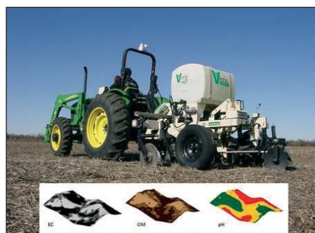
Obr. 11: Platforma MSP3 – Veris Technologies ( www.veristech.com ).
